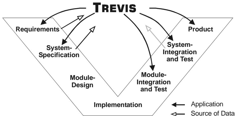
Fig. 1: V model describing the different phases of a development process.
